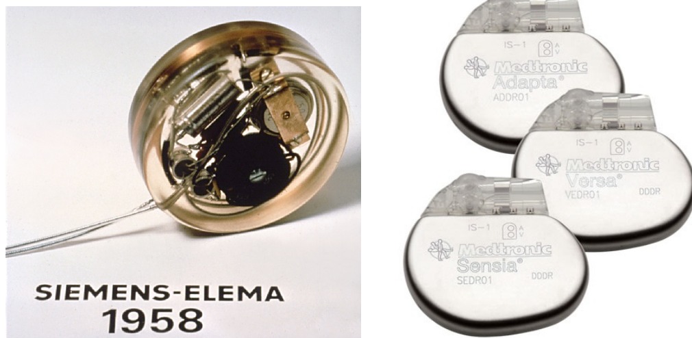
(a) The original pacemaker developed by engineer, Dr. Rune Elmquist, in conjunction with Siemens, for Arne Larsson. This version of the cardiac pacemaker was encapsulated in epoxy resin in a plastic cup, and failed within a few hours.[29]
