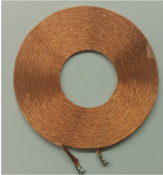
Figure 4.18: Commercially available, machine wound, single layer, wireless power delivery coil embedded within a smartphone.
