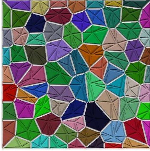
Figure 5.1: Voronoi mesh generated for points on the unit square.
