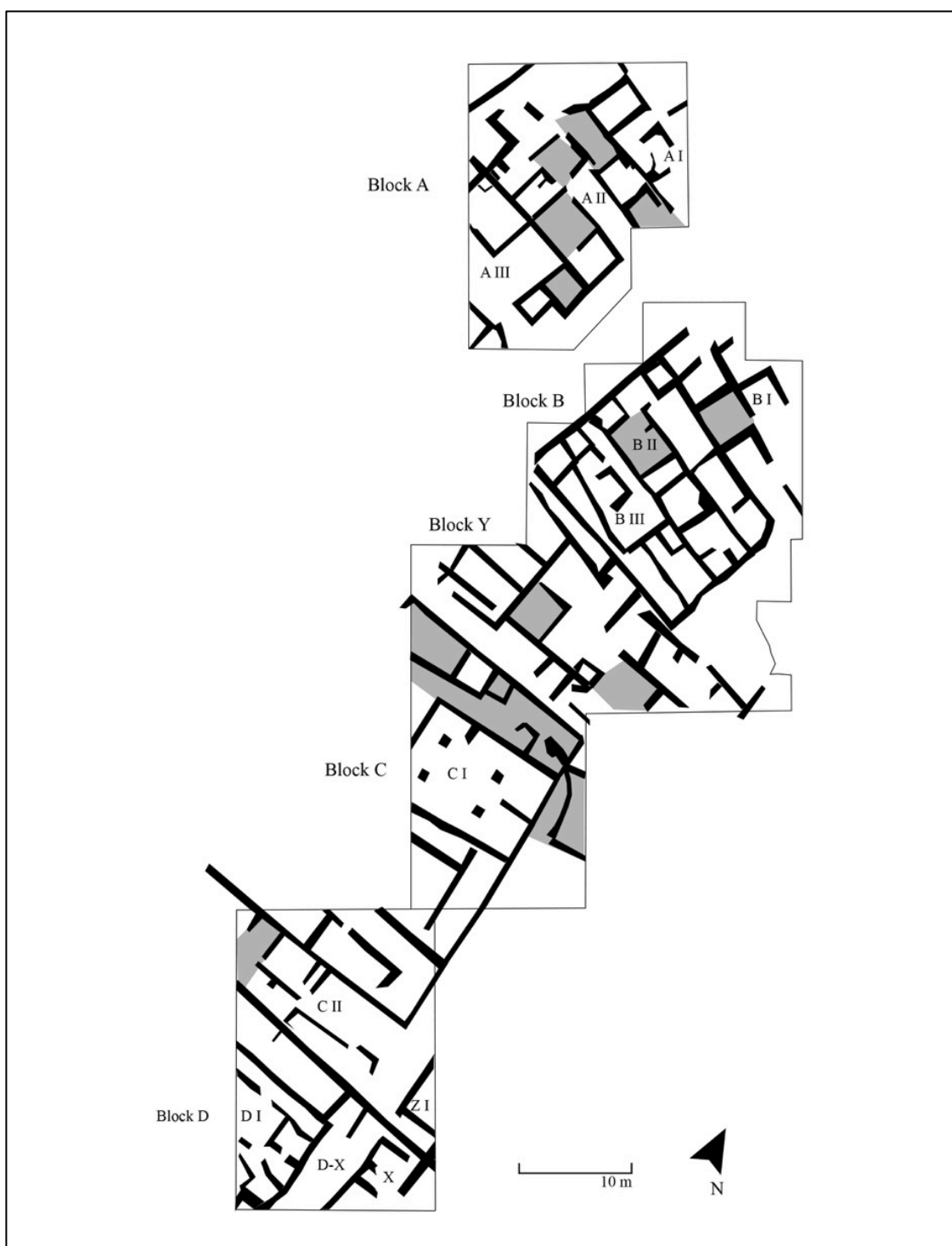
Figure 6.9 Excavated plan of La Loba settlement with areas in grey showing the presence of tubes ( tubuli ) of spuma argenti or litharge from lead metallurgy that forms in the course of cupellation (after Figure 43 in Domergue & Tollon 2002: 72).
