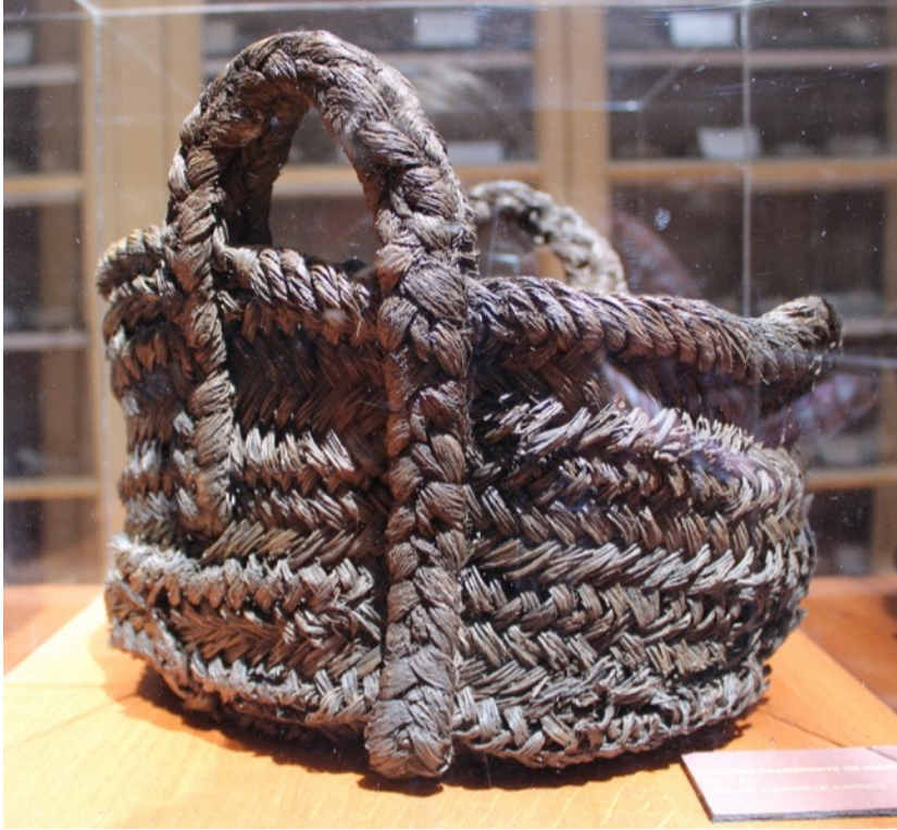
Figure 7.17 Esparto-grass basket from Algarés, Aljustrel for lifting ore and other material out of mining shafts (author photo, Museu Geológico, Lisbon).
