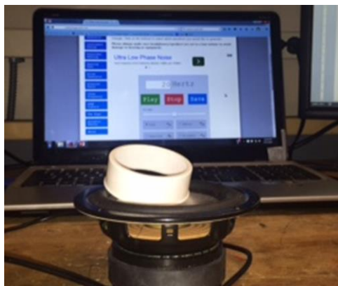
Figure A.3.1 A circular boundary condition is shown in the image sitting on top of a speaker. A laptop with a frequency generator application is in the background.
