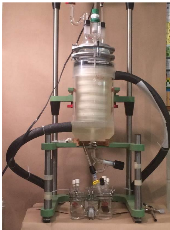
Figure 5.1 Batch reactor constructed for the formation of the clathrate electrolyte solution. The inner chamber contains a helical Teflon structure used to continuously stir the electrolyte solution. The entire vessel is gas tight and placed under CO 2 pressure slightly above 1 atm. The reactor is also water jacketed for temperature control 71 .
