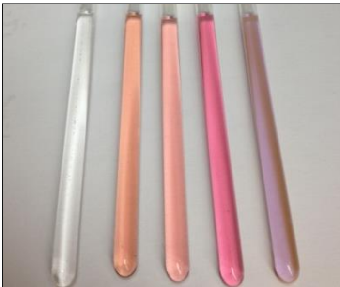
Figure 3.9 Gold nanoparticle suspensions. The gold particles have diameters of 2 nm, 5 nm, 10 nm, 50 nm and 100 nm from left to right. The difference in color is due to the change in surface plasmon resonance with particle diameter 55 .
