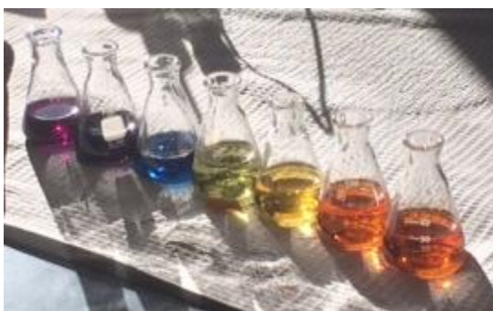
Figure A.3.4 Nanoparticle solutions produced by students during the execution of the laboratory. The analytical balances were not leveled prior to the experiment so the small mass of reducing agent required for the synthesis was inaccurately measured and produced a variety of nanoparticles as seen by their different plasmon resonances.
