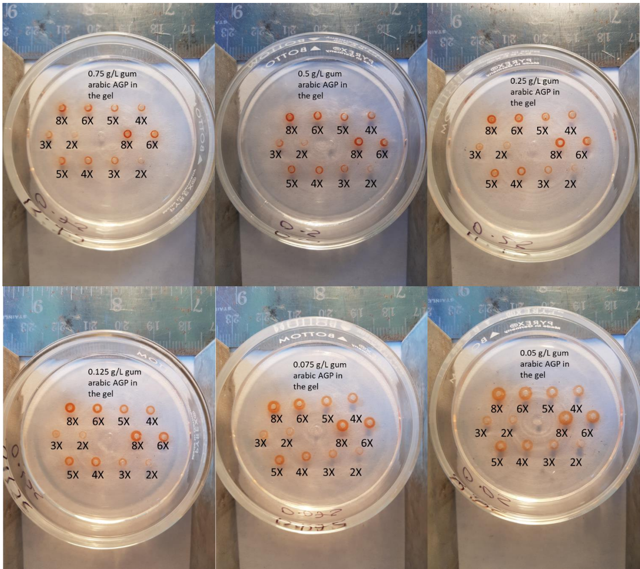
'Reverse' gel assay optimization process; \beta DGlc (1) in the wells, concentrations ranging from 2X to 8X where X=0.13 mM
