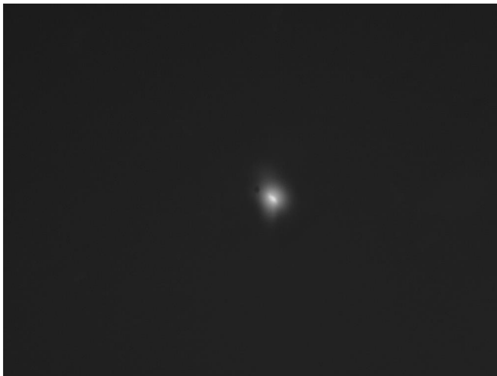
Figure 3.24 The X-ray laser overlapping imaged by YAG Screen fluorescence. The larger spot is laser and the smaller, brighter spot in the center is the X-ray spot.
