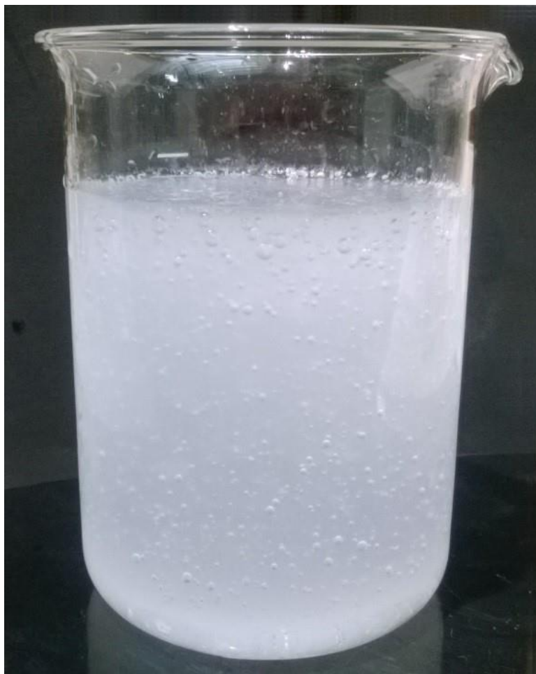
Figure 7.2 Picture of Clathrate Hydrates made with the bath reactor.
