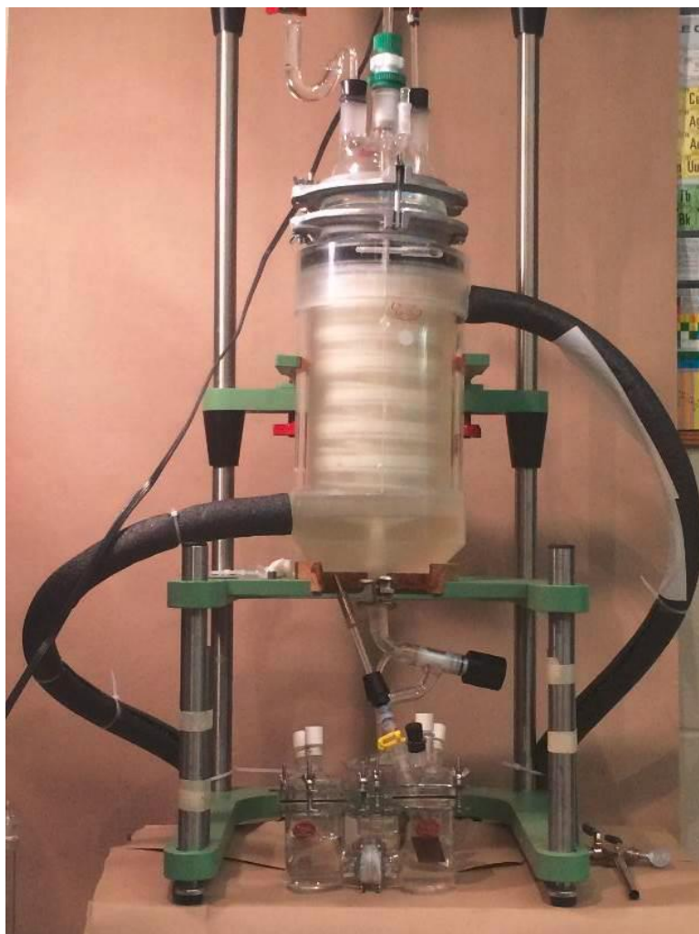
Figure 7.1 Batch reactor constructed for making the clathrate electrolyte solution. The inner chamber contains a helical Teflon pedal that continuously stir the electrolyte solution. The entire vessel is gas tight and placed under CO 2 pressure slightly higher than 1 atm. The whole system temperature was controlled by a chiller to be constantly 2°C.
