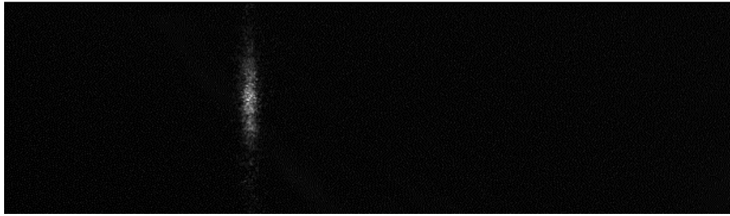
Figure 3.15 Streaked UV pulse, shown as a vertical line on the image. The position of this vertical line is a reflection of Timing of the pulse.
