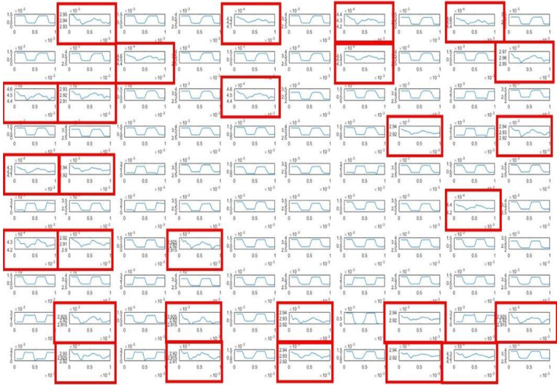
Figure 4.7: The 32 channel connector is grounded, showing attenuated signals on connected channels only.
