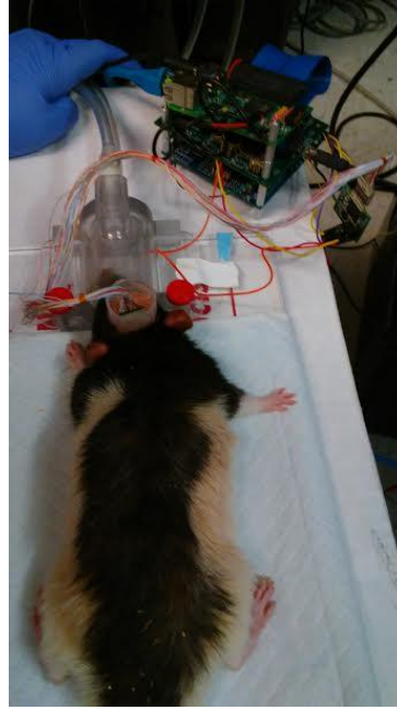
Figure 4.14: Animal experimental setup with Utah MEA connected to Impedance Spectroscopy Test system through a multi-channel cable connector.
