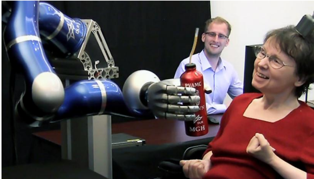
Figure 1.2: A Brain gate subject using spike-activity from motor cortex (M1) to manipulate a robotic arm carrying a water bottle to the appropriate position for the subject to drink from it [7].
