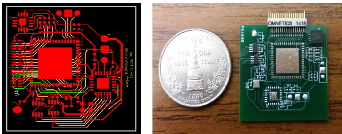
Figure 4.2: 32-channel Impedance Spectroscopy Prototype System PCB layout and fabricated board.
