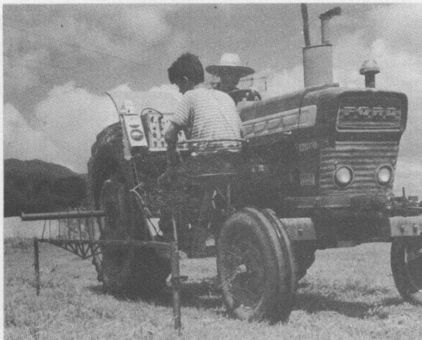
Fig. 9 Set-up of depth measuring device for tractor mobility studies.
