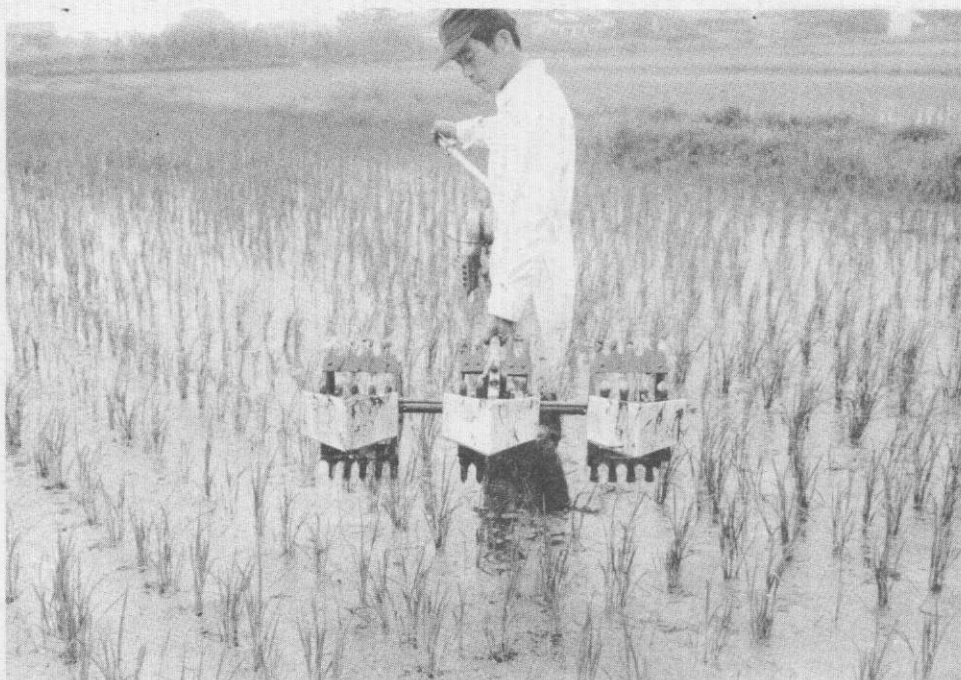
Fig. 1 Power weeder manufactured in Japan by Ohtake Nouki Seisakusho Co., Ltd. based on the IRRI concept.
