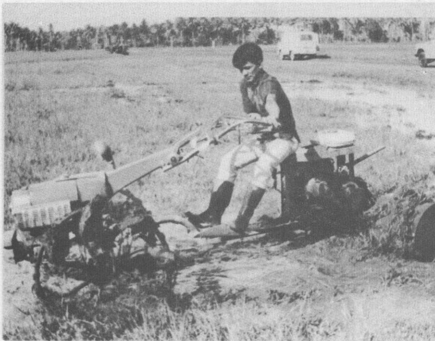
Fig. 6 Dual tractor set-up for tiller wheel tests.
