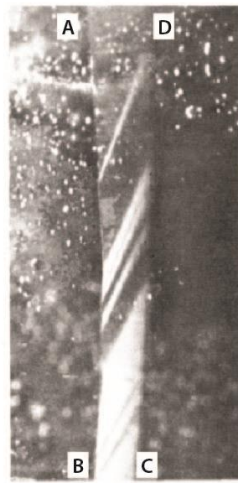
Figure 3: (a) Faceting along the grain boundary in an ice bicrystal, photographed in transmitted light (left) and drawn schematically (right). The image is looking down on a boundary inclined relative to the page. The actual boundary width (BC) is \sim 5 mm. Reproduced from Hondoh & Higashi (1983). During these authors' study, 34^\circ tild boundaries in ice bicrystals were subjected to shear stress of \sim 100 kPa. They have interpreted the variations of refracted light along the grain boundary to be facets with orientations varying as in the sketch. (b) Schematic interpretation of the structure of grain boundaries during deformation of polycrystalline ice (Caswell et al., 2015). GBDs (light-dashed lines) are able to glide along facets but pile up at facet intersections (heavy-dashed lines). Stress concentrations due to these pileups cause emission of lattice dislocations, which relieve pileup stresses and allow sliding to continue; thus, grain boundary structure plays a first-order role in GBS in ice.
