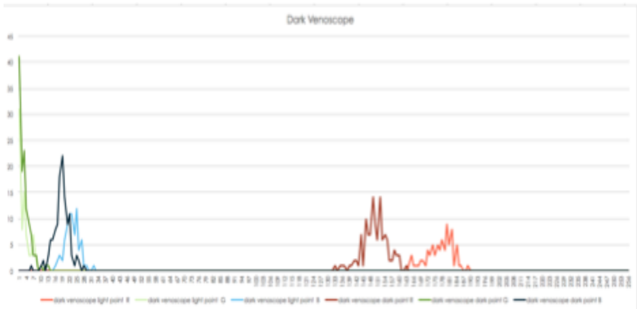
Figure 4: RGB graphs derived from Venoscope. The distance between red and orange peaks represents the contrast.
