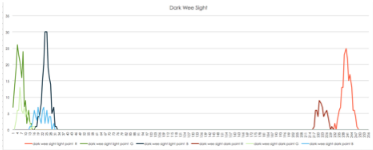
Figure 5: RGB graphs derive from the WeeSight. The distance between red and orange peaks represents contrast.
