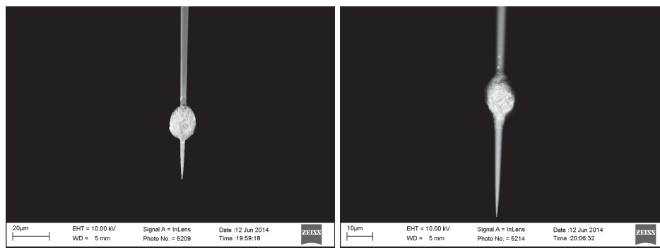
Fig. 4.2 Salt buildup present on tips that have been electro sprayed with voltages approximately 3 times greater than their onset voltages.
