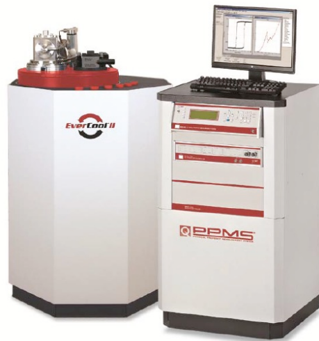
Figure 2.8 The real image of PPMS including the sample chamber and controller station only (from PPMS manual).
