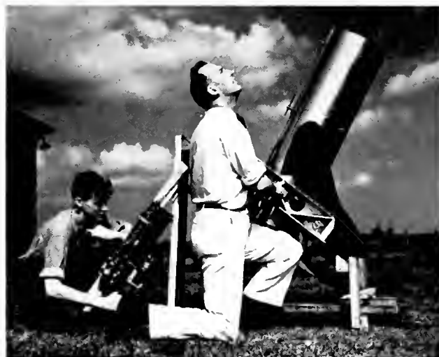
ASTRONOMICAL HOWITZER that went to Brazil with Prof. Charles H. Smiley and Arthur A. Hoag '41 on the Brown University 1940 Solar Eclipse Expedition. THE COVER PHOTO shows them looking into the case of this unique Schwarzschild camera, first of its kind ever to be used for eclipse photography.
