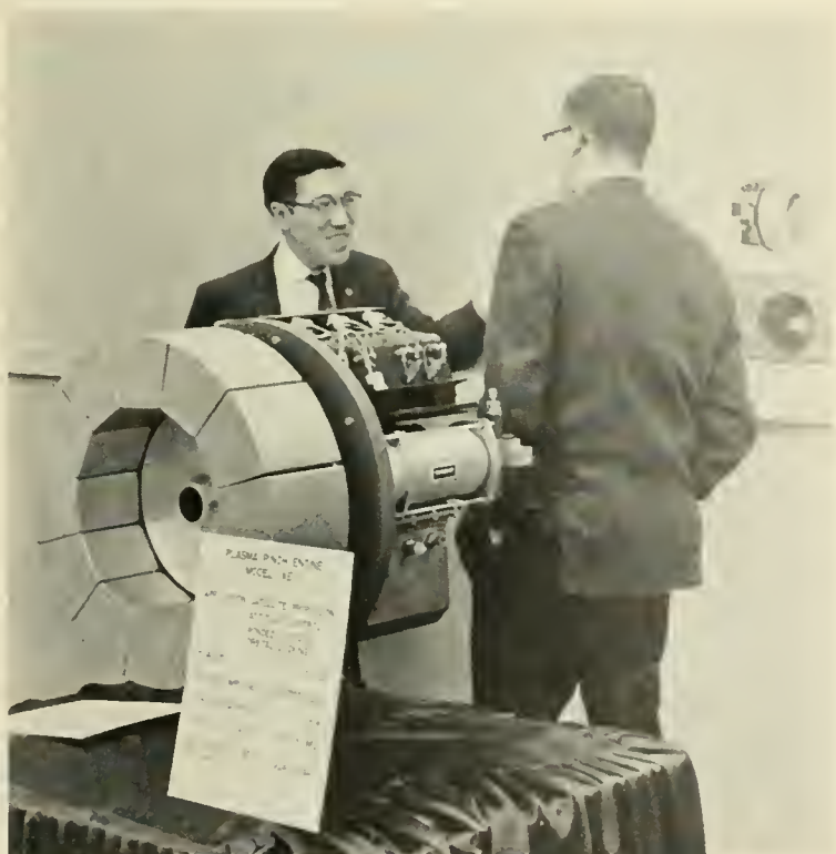
PROPULSION DEVICE, at left, was for a space project. The plasma pinch engine was designed for satellite propulsion, attitude control, rendezvous, and orbital docking.
