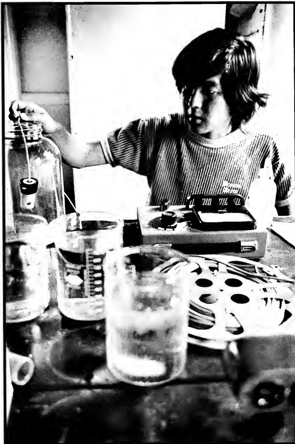
Ray Moriyasu operates an oxygen meter borrowed for the duration of the project from Rhode Island Junior College. He is conducting part of a 20-day biochemical oxygen demand test, which measures the rate of oxygen depletion over that period of time.
