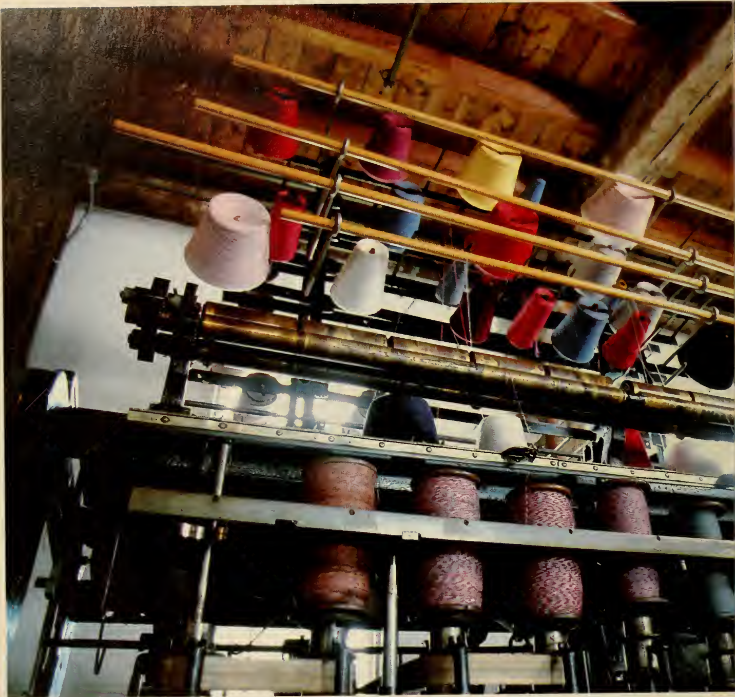
The Slater Mill exhibits a variety of machines used in the production of cotton, including this ring spinning machine.
