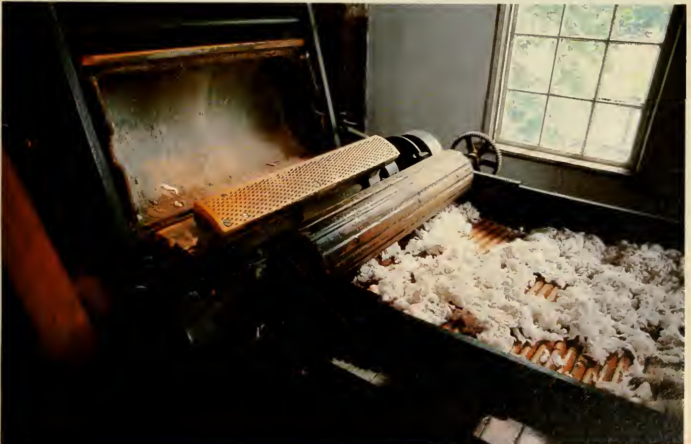
A breaker and picker on display in Slater Mill. This machine would break the cotton apart, and cull the seeds from the raw fiber.
