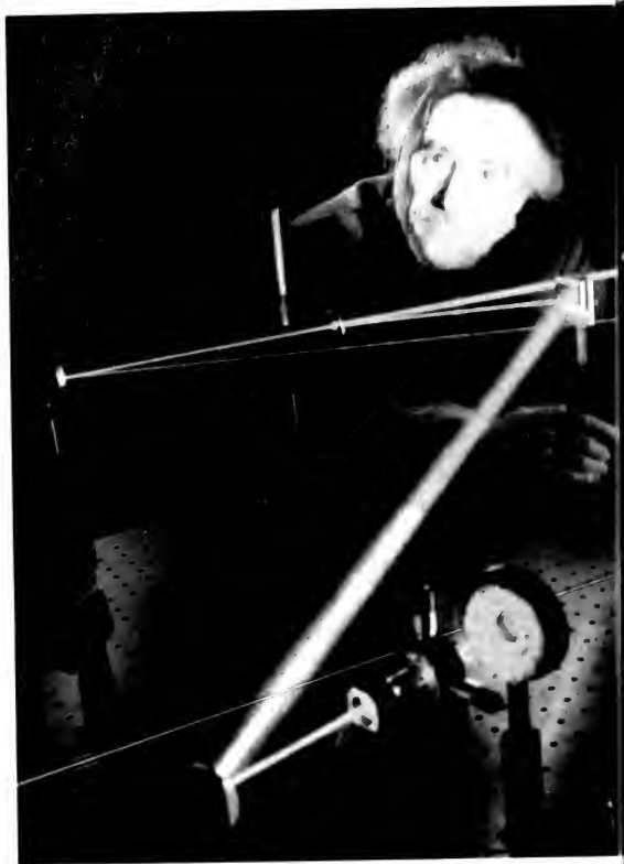
A WIZARD AND HIS MAGICAL LIGHT BEAMS: Hendrik Gerritsen demonstrates two of the lasers in his laboratory. The red laser beam, emanating from a device out of camera range on the right, becomes two half-beams after passing through a beam splitter. One half-beam bounces off the mirror in Gerritsen's hand, is directed to another mirror at lower left, and is sent through a lens and an "iris" to project the circle of reddish light, at right. The other half-beam strikes a mirror, left, and is directed to a point on the circle of red light.
