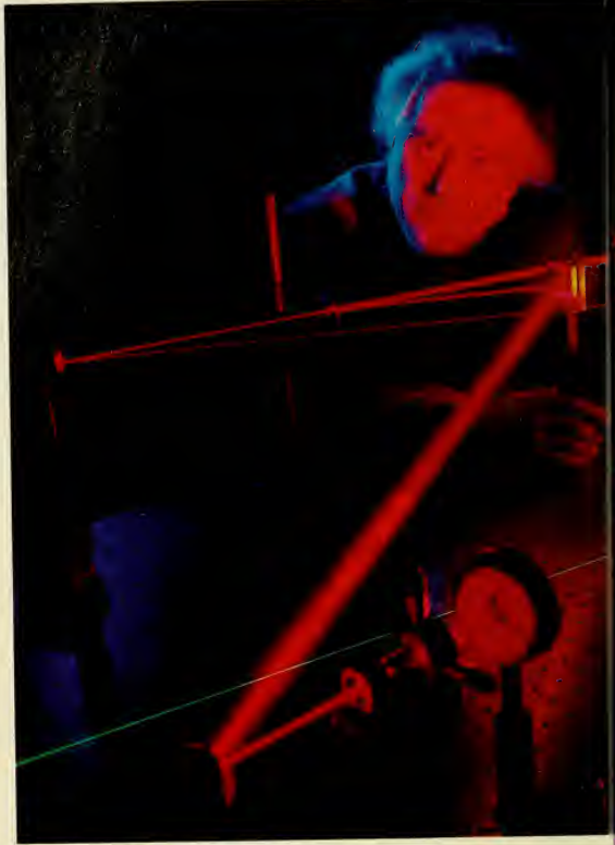
A WIZARD AND HIS MAGICAL LIGHT BEAMS: Hendrik Gerritsen demonstrates two of the lasers in his laboratory. The red laser beam, emanating from a device out of camera range on the right, becomes two half-beams after passing through a beam splitter. One half-beam bounces off the mirror in Gerritsen's hand, is directed to another mirror at lower left, and is sent through a lens and an "iris" to project the circle of reddish light, at right. The other half-beam strikes a mirror, left, and is directed to a point on the circle of red light.
