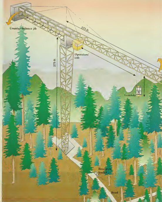
The Wind River Canopy Crane. Located sixty-five miles northeast of Portland, Oregon, the crane and its gondola allow canopy scientists to study the temperate rain forest in a more systematic and exact way – without risking life and limb on thin ropes and swaying branches.
