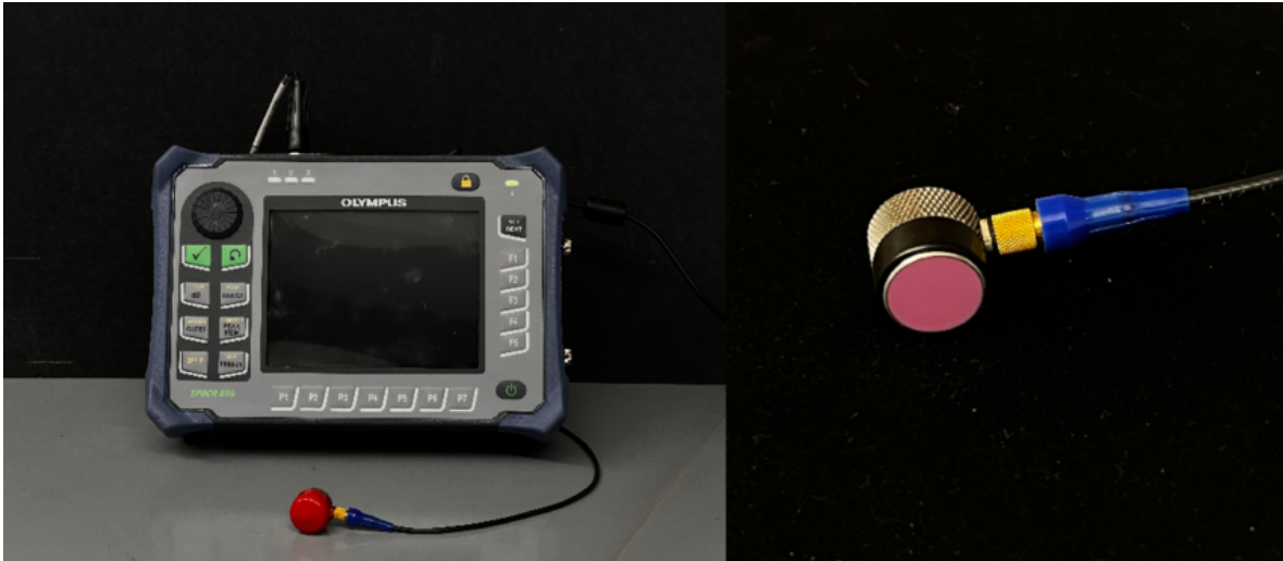
Figure 3: Olympus EPOCH 650 (a NDT) flaw detector and 1 MHz probe.
