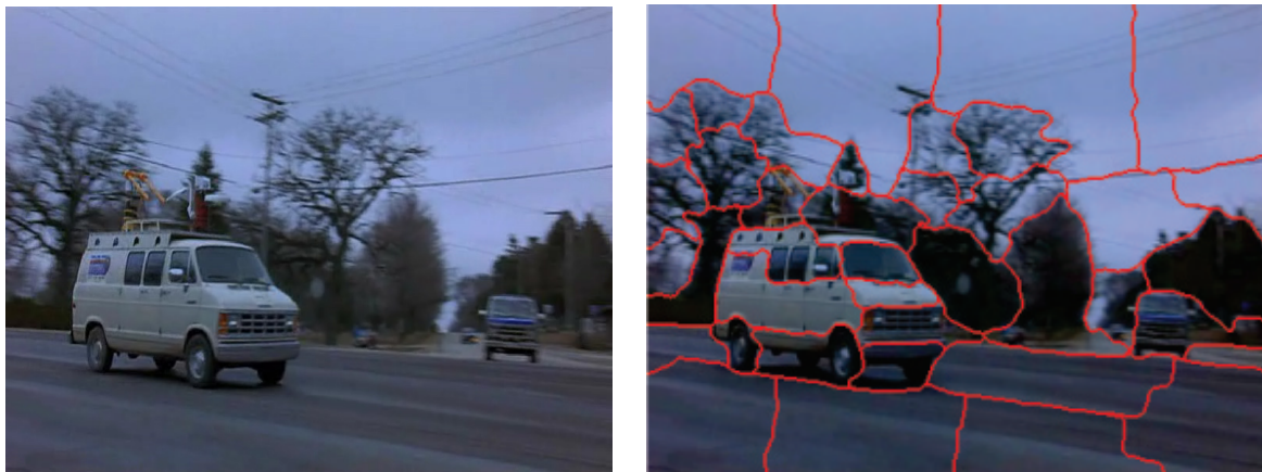
Figure 1.1: This figure shows the segmentation of the figure on the left using implementation based on [75, 65]. Note how the segmentation is far from the desired segmentation as the whole van.
