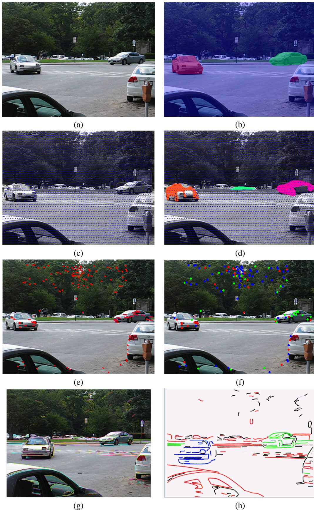
Figure 6.2: The goal of motion segmentation is the delineation of moving objects relative to a background from the sequences of frames in a video. A frame of a video is shown in (a) and the ideal results are depicted in (b). (c) dense optical flow estimation and (d) segmentation into component based on fitting a parametric 2D motion model, shown in pink, green and orange. (e) KLT features and (f) factorization based segmentation shown in red, green and blue. (g) curves superimposed on the image and (h) segmentation based on affine motion model where distinct
