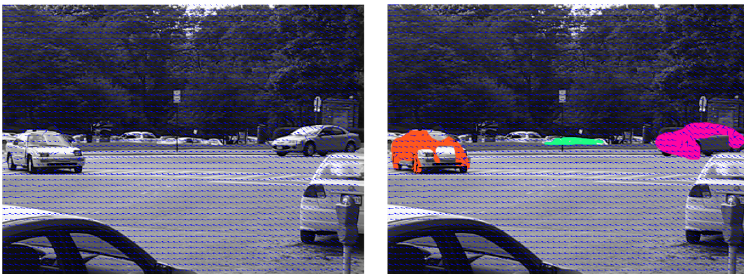
Figure 1.4: This figure shows the motion segmentation using dense-flow computed on pixels. The left image shows dense flow estimated on each pixel and the right shows segmentation of regions based on their flow into different motions shown in different colors namely green, pink, and orange.
