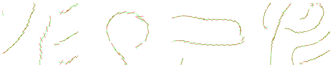
Figure 6.6: The third-order edge [88] detector (shown in green) provides a better estimate of edge-orientation as compared to traditional operators (shown in red).
