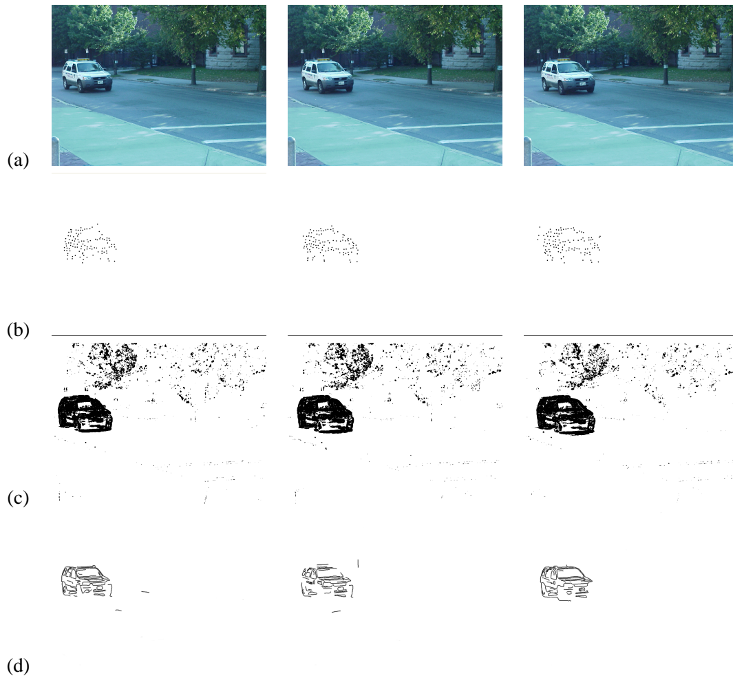
Figure 5.2: This figure shows the motion segmentations from different approaches. (a) Three frames of an outdoor video sequence and the motion segmentation of this video sequence using (b) KLT features based segmentation, (c) region based segmentation and (d) its curve-based object segmentation [48] is shown. Note how all these segmentation have noise and missing gaps.
