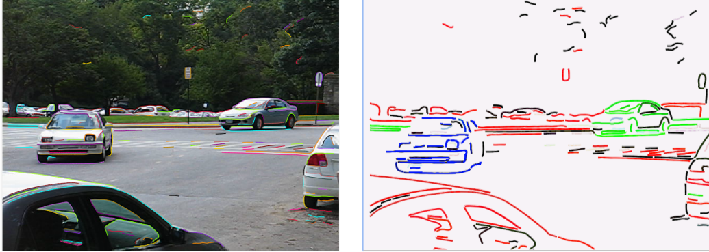
Figure 1.5: This figure shows the motion segmentation using curves . The left image shows curves and the right shows segmentation of curves into different motions shown in different colors namely green, blue , and red. The black color curves do not belong to any group.
