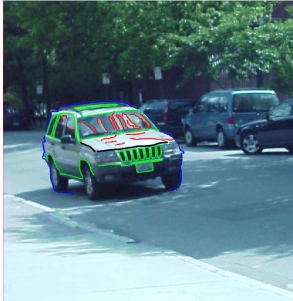
Figure 1.10: This figure classifies curves into different categories into (i) reflectance curve (green) due to reflectance discontinuity, (ii) occluding contour (blue) due to depth discontinuity, (iii) high-light contours (red) and (iv) ridges due to surface discontinuity.
