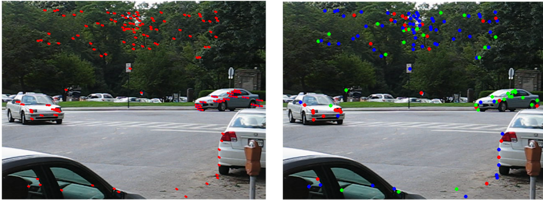
Figure 1.3: This figure shows the motion segmentation using features. The left image shows tracking of features and the right shows segmentation of features into different motions shown in different colors namely green, red, and blue.
