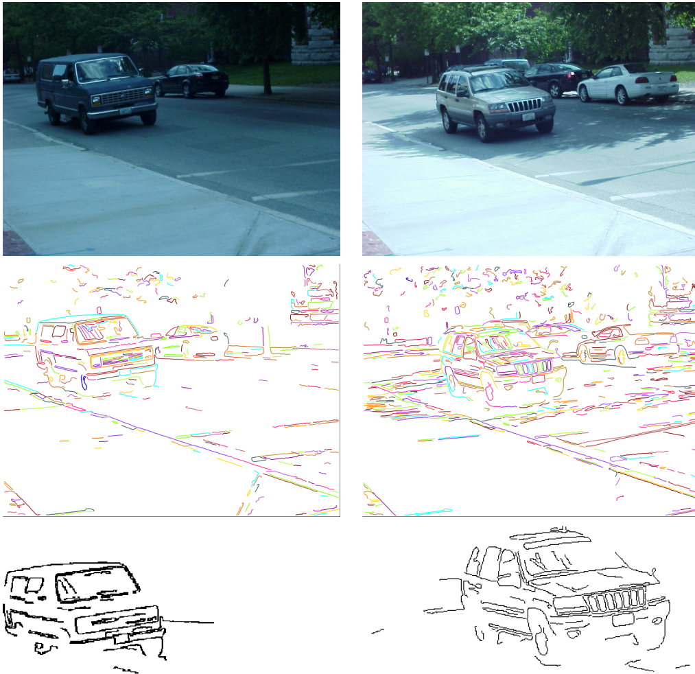
Figure 3.13: Results of Figure-ground segregation based on two adjacent frames for a Van (first frame shown on the left) and an SUV(first frame shown on the right). The top row shows the original image, the second row shows the contours extracted and last row shows the segmented object.
