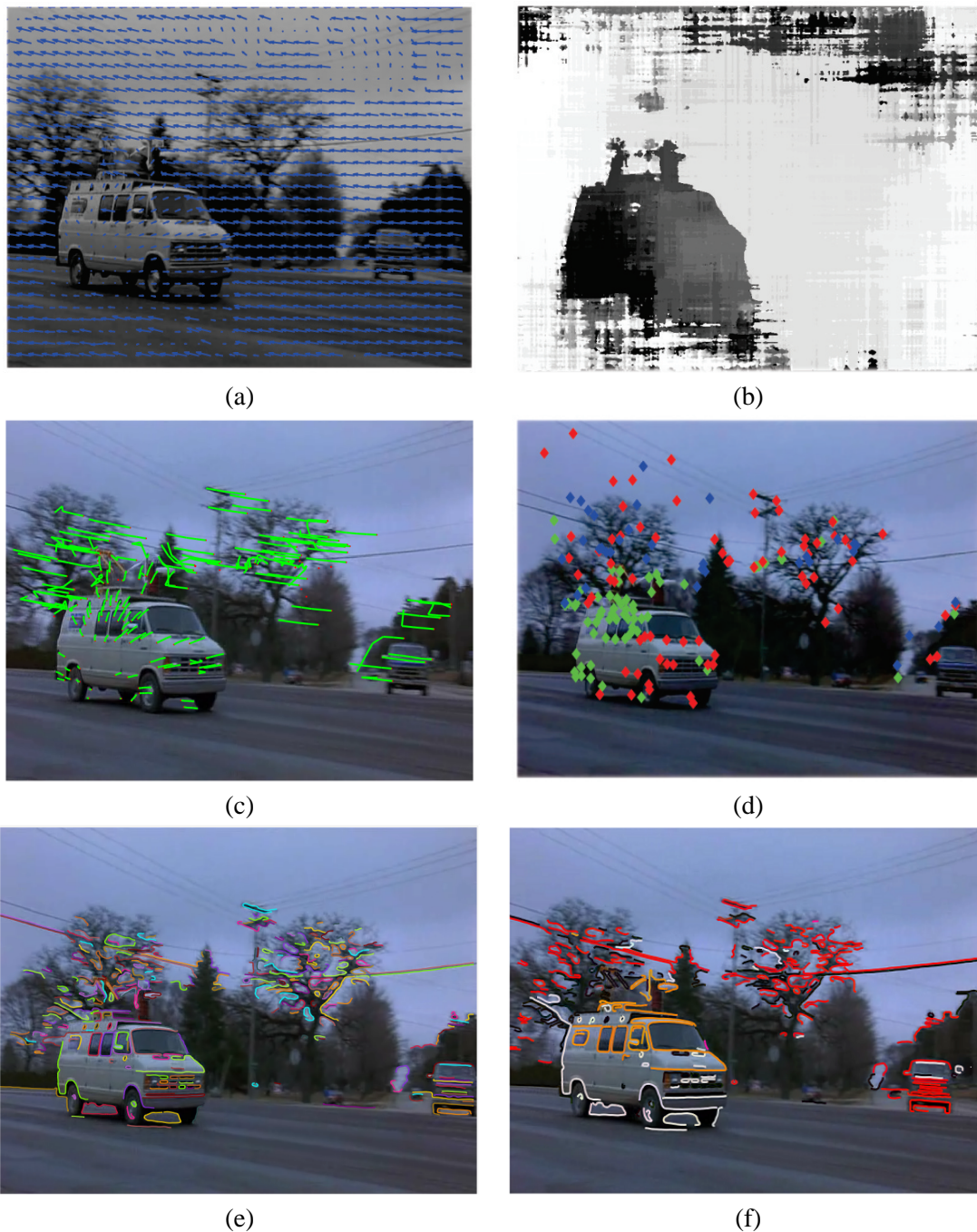
Figure 6.3: (a) A frame from the movie “Groundhog Day” with optical flow superimposed on it. (b) the frame can then be segmented based on 2D parametric motion models and the resulting segmentation. This clearly shows the van is divided into two pieces. Similarly the tracked KLT features of the same frame are shown in (c) and a factorization-based segmentation of these features is shown in (d), where each color represents a different group. Clearly, the van’s features are grouped in the different segments, one of which shares features from background. Finally, the curves on the van (e) are tracked and segmented based on the similarity of 2D motion using an affine model. The resulting segmentation in (f) clearly shows that the van is segmented into two regions.
