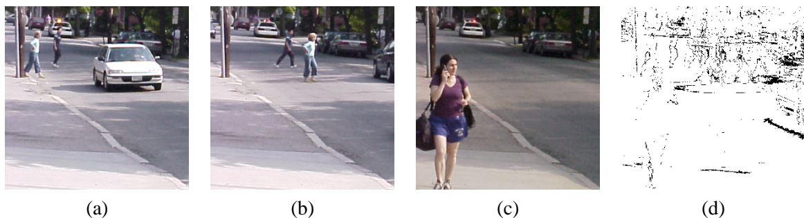
Figure 4.1: The effect of sudden illumination change on intensity-based background modeling . (a,b) a pair of typical background images,(c) a frame when the illumination has changed and (d) the corresponding foreground detection. Observe that the foreground, the pedestrian, has not been identified and a large part of the background is labeled as the foreground.
