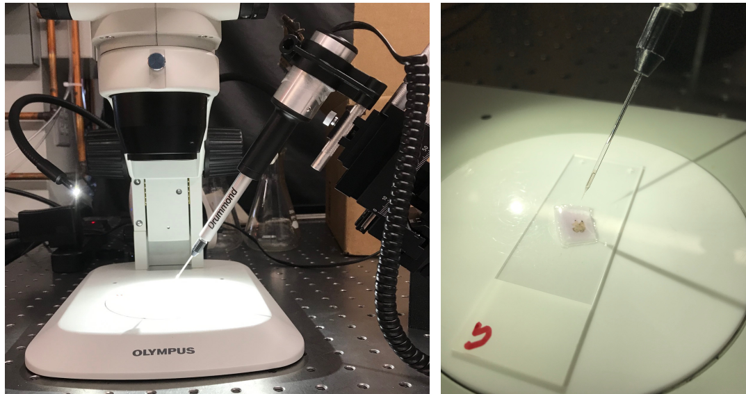
Figure 16 Image of nano-injector setup. (Left) Shows typical injection setup under visualization of microscope, (Right) S-ILM injection on retinal-flat mount .
