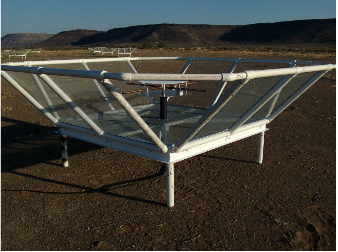
FIGURE 3.1: A single dual-polarization dipole antenna from the Donald C. Backer Precision Array for Probing the Epoch of Reionization. The wire mesh reflectors decrease the response to sources from the horizon. The stage of the PAPER array used for the analysis in this chapter was composed of 64 of these dipole antenna.
