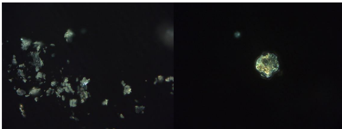
Figure 49. Sections of microspheres of 5% w/v PMMA:PCL = 3:7 with polarized light at 40x magnification
