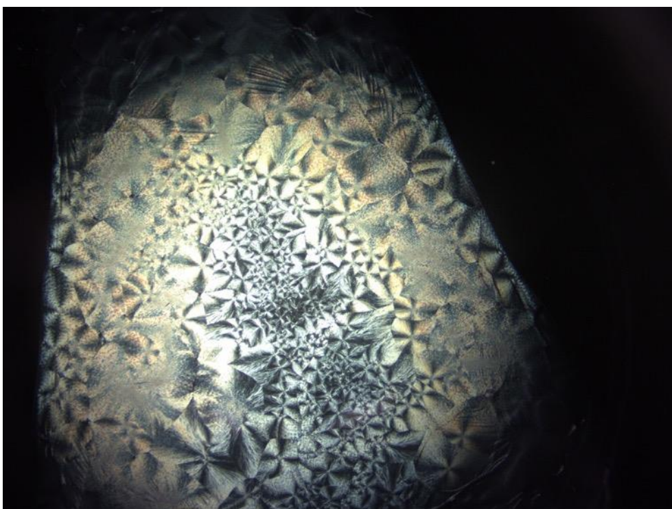
Appendix 2. Film Cast of 20% w/v PMMA:PCL = 3:7 at 4x magnification with polarized light
