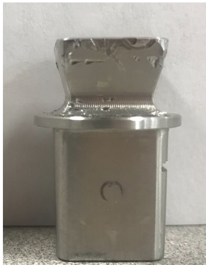
Figure 3.23: Metal Pyramidal Connector insert for the proximal piece
