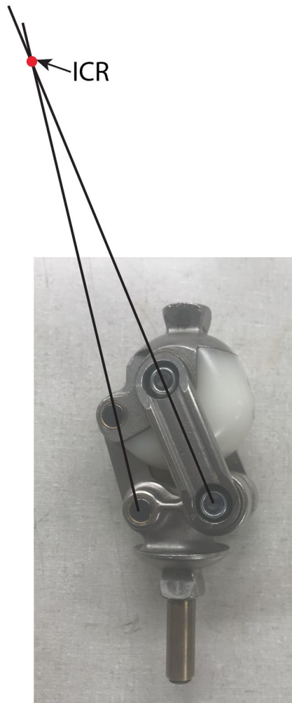
Figure 3.15: ICR of a 4-Bar Knee (Ottobock Titan)
