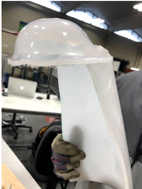
Figure 2.18: Heat fusing the cup section with the backbone required reaching right below the melting point and pressing the two pieces together
