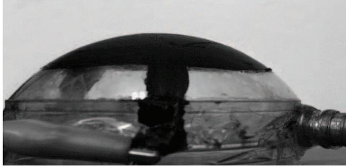
**Figure 4.1:** The benchtop membrane pressurization set-up, showing a membrane at an intermediate stretch. The compliant electrode, made from carbon grease, is seen on the surface of the transparent membrane.
