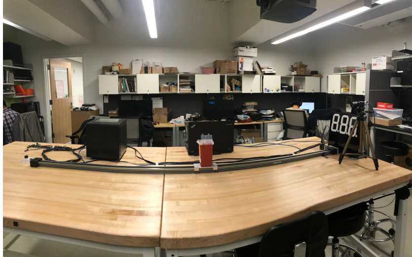
Figure 12: Full EEG, conveyor belt, laptop, video camera, dial, and rating screen setup
