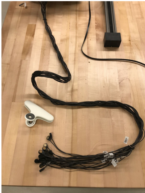
Figure 10: Tripolar Electrodes, labeled and the clip used to attach the wires to the back of the participant's shirt
