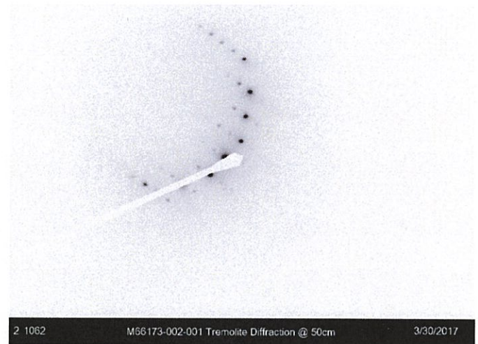
Figure 13a. TEM Image of a tremolite fiber and diffraction pattern in sample M66173-002.
