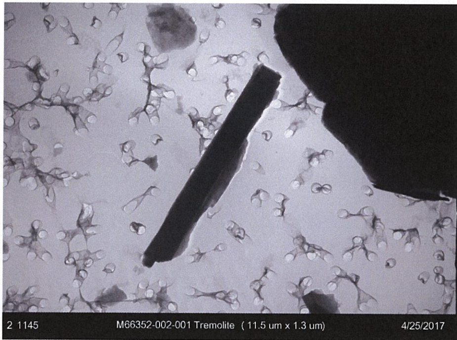
Figure 15a. TEM image of a tremolite fiber in Sample M66352-002.
