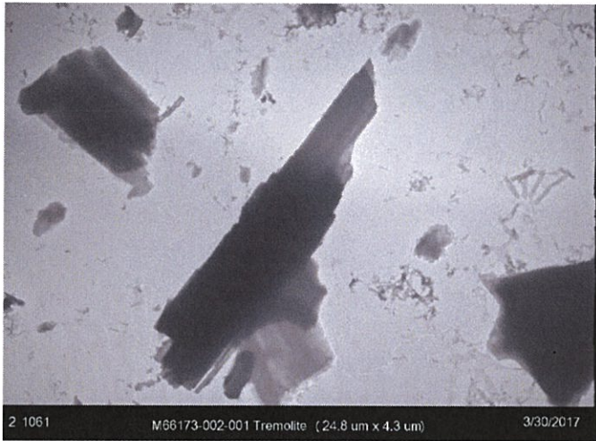
Figure 13a. TEM Image of a tremolite fiber and diffraction pattern in sample M66173-002.
