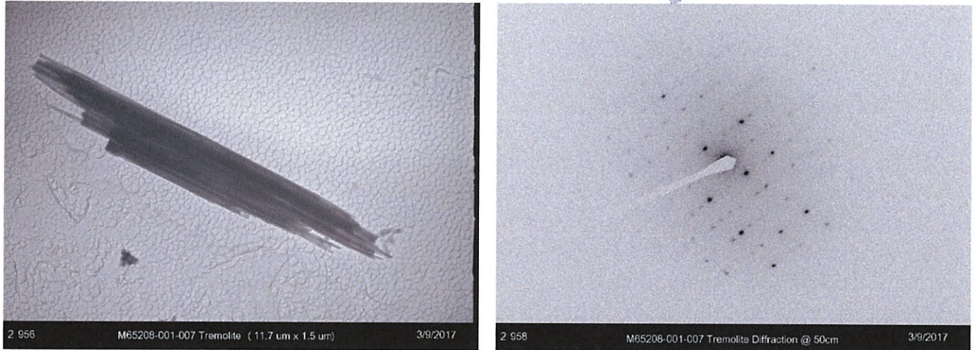
Figure 9a. TEM Image of a tremolite bundle and diffraction pattern in sample M65208-001
