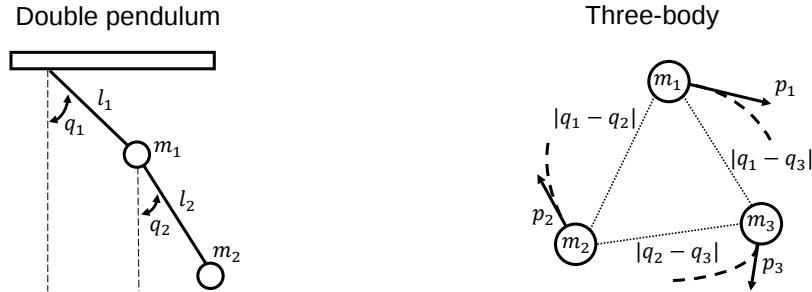
Figure 2.5: Illustrations for the double pendulum and the three-body. (Left) The double pendulum system consists of a pendulum attached directly to another one. The i -th pendulum is made of a ball of mass m_i connected to a massless rigid rod of length l_i . (Right) The three-body system consists of three planets of mass m_i , the motion of which is governed purely by gravitational force.
