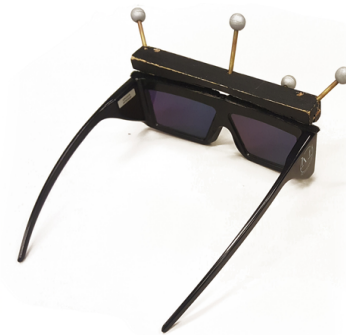
(b) The CAVE B environment located at Brown University. It uses optically tracked CrystalEyes stereo shutter glasses.
