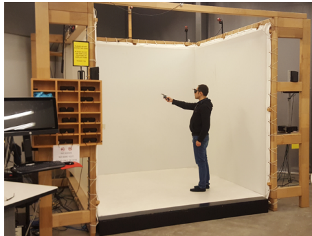
(b) The CAVE B environment located at Brown University. It uses optically tracked CrystalEyes stereo shutter glasses.
