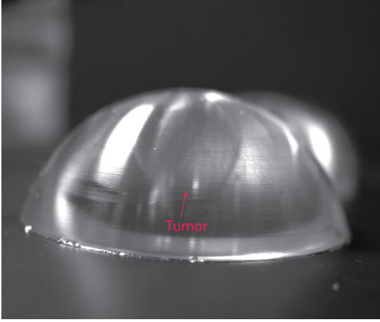
Figure 12: PDMS breast with a 2 cm tumor inside. Figure 13: Applying Olympus 1 ultrasound machine to the PDMS breast.
