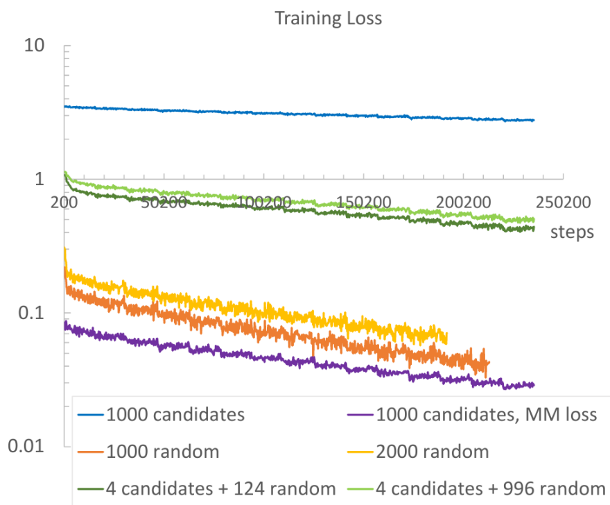
Figure B.2: Evolution of the loss on the training set, as training of BM25→CODER(RepBERT) progresses. Different curves correspond to a different type and number of documents used as negatives during training. While training loss is decreasing in all cases, only using numerous retrieved candidates as negatives, combined with a list-wise KL-divergence loss, results in a significant improvement of performance over the base method (see Figure 2.4) on the validation and test sets.
