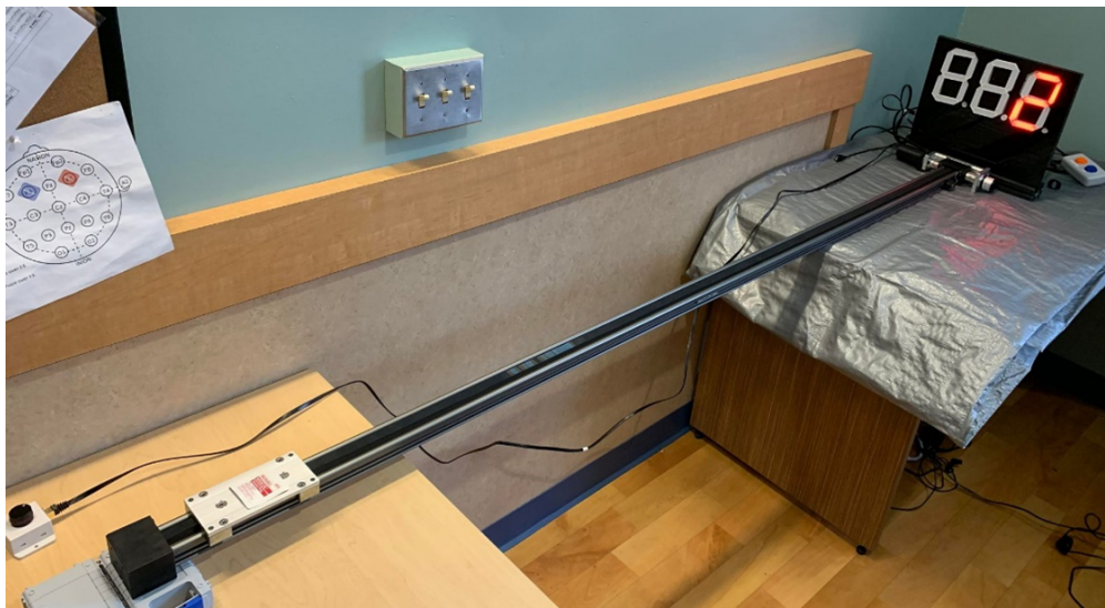
Figure 5: Conveyor Belt PROVOC setup with caddy extended to Position 5 (closest to the participant). Hand dial is used to enter SUDS ratings, which are shown on the display.
