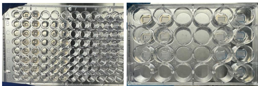
Figure B.1.: Agarose mold for 96 well plate and 24 well plate microarray
