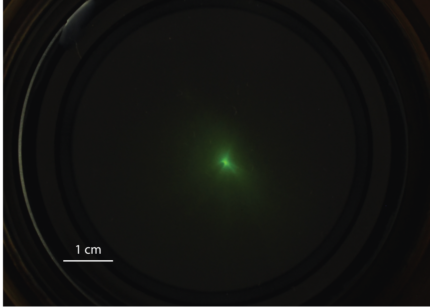
Figure 2.3.6: MCP image of focused ion beam. Photograph of the MCP screen showing a well-focused ion beam.
