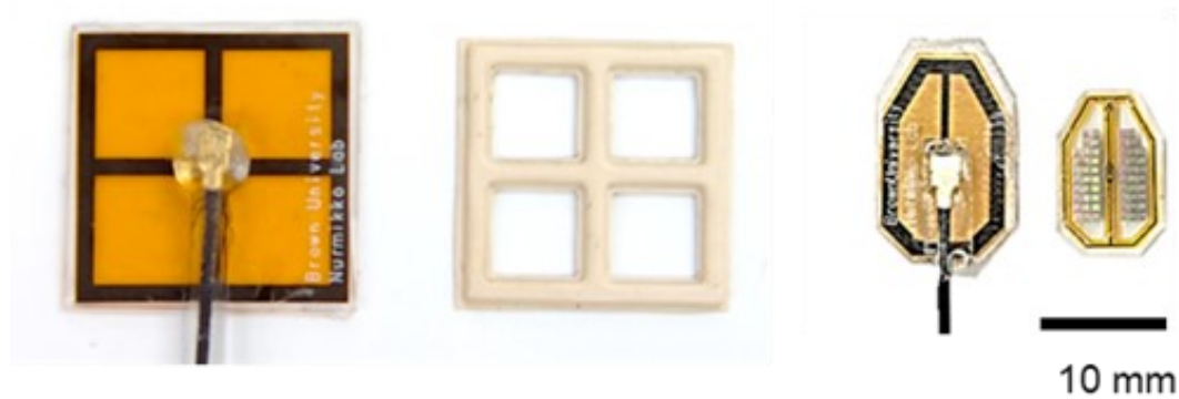
Figure 5-12. (left) The Tx and relay coil for the (proposed) primate model packaged with PDMS or LCP. (right) The Tx and relay coil for the (implemented) rodent/rat model. The relay coil was packaged along with a set of 56 individually addressable neurograin chips.
