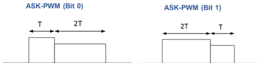
Figure 2-5. Sample ASK-PWM bits for data and frame synchronization; a “short high” represents bit 0 (left) while a “long high” is equivalent to bit 1 (right).
