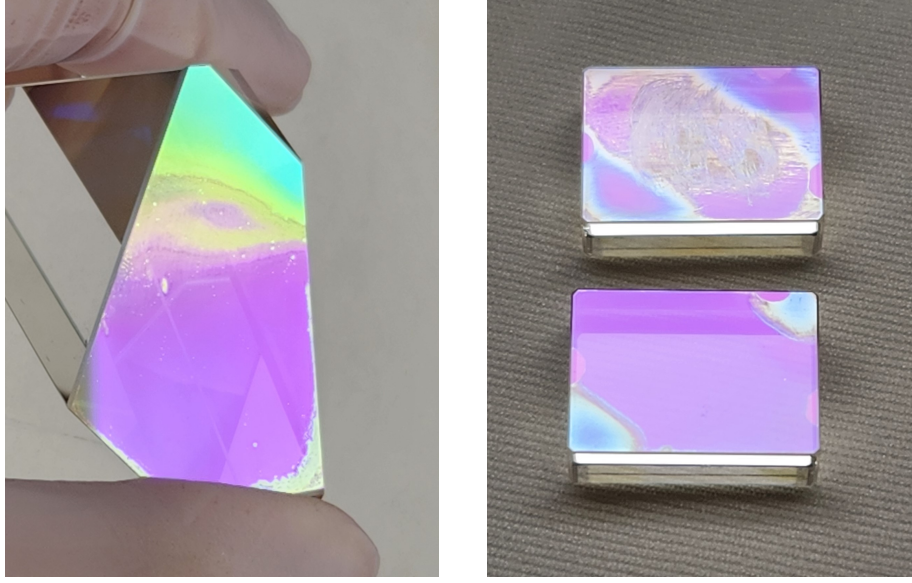
Figure 4.21: Degraded HR surfaces of the Raman corner cube (left) and two of the MOT mirrors (right). The surface degradation is illuminated by shining white light on the surface at a particular angle of incidence.
