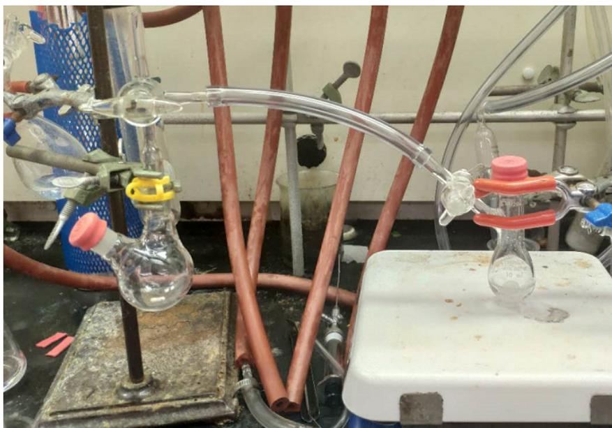
**Figure 5.5** Set up for hydrogen sulfide detection using turn-on fluorescence sensor *C7Az*.
