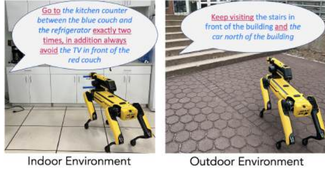
Figure 1.5: Lang2LTL-2 grounds spatiotemporal navigation commands in indoor and outdoor environments. The spatial and temporal components of the example commands are highlighted in blue and red, respectively.
