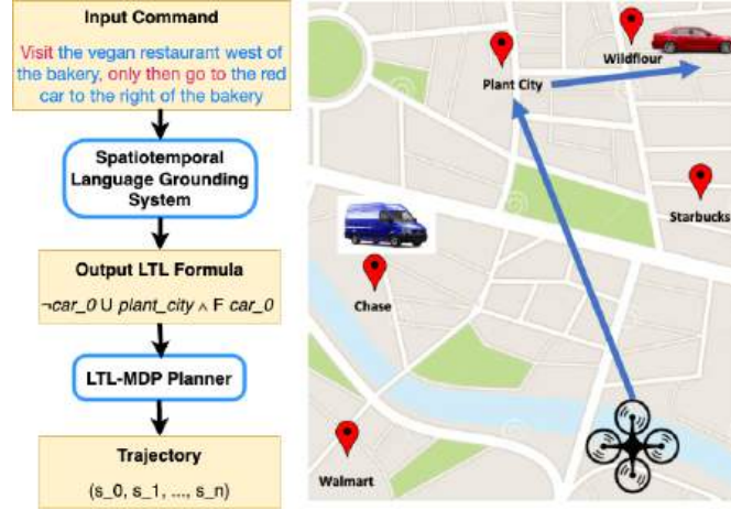
Figure 4.2: An example of an input spatiotemporal navigation command whose spatial and temporal components are highlighted in blue and red, respectively, an output LTL formula whose propositions are grounded to physical landmarks, and an execution trajectory in the environment.
