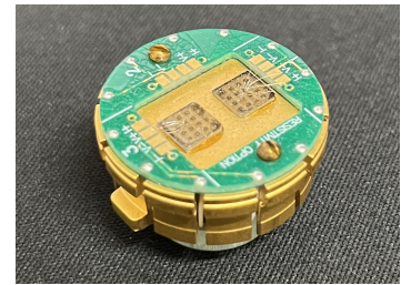
Figure 17: PPMS resistivity sample chuck. Image shows 2 separate bonded samples.
