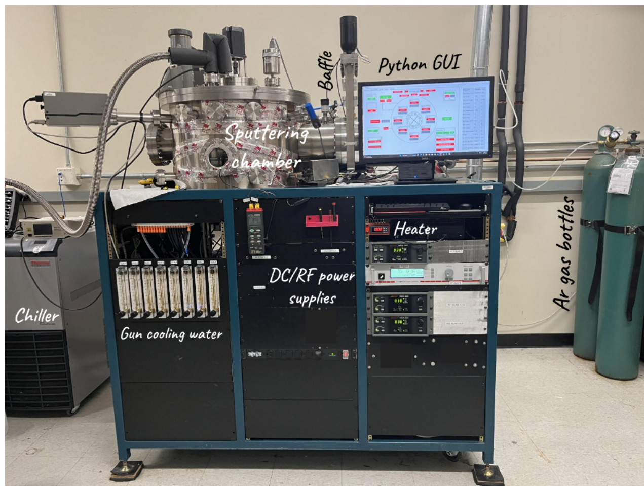
Figure 8: Magnetron sputtering system used for sample fabrication. Important components are labeled.
