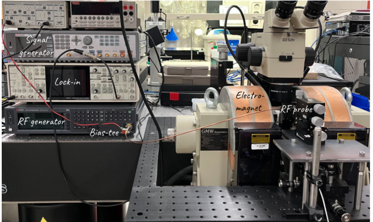
Figure 23: Ferromagnetic resonance measurement setup. Important components are labeled.
