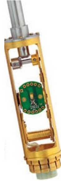
Figure 18: PPMS resistivity rotator mount used for angle-dependent R_{xx} measurements.
