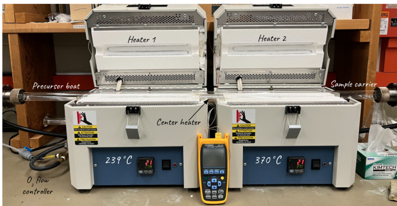
Figure 9: Chemical vapor deposition system used for epitaxial sample fabrication. Important components are labeled. \text{O}_2 bottle not pictured.
