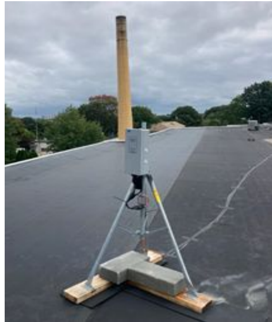
Above: Breathe Providence's BEACO2N monitors (left) and the Community Noise Lab's Optimus + Red Class 1 sound level meters (right)
