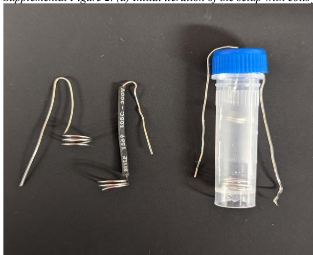
Supplemental Figure 2. (a) Initial iteration of the setup with coils for electrodes; (b) Secondary iteration of the device with
