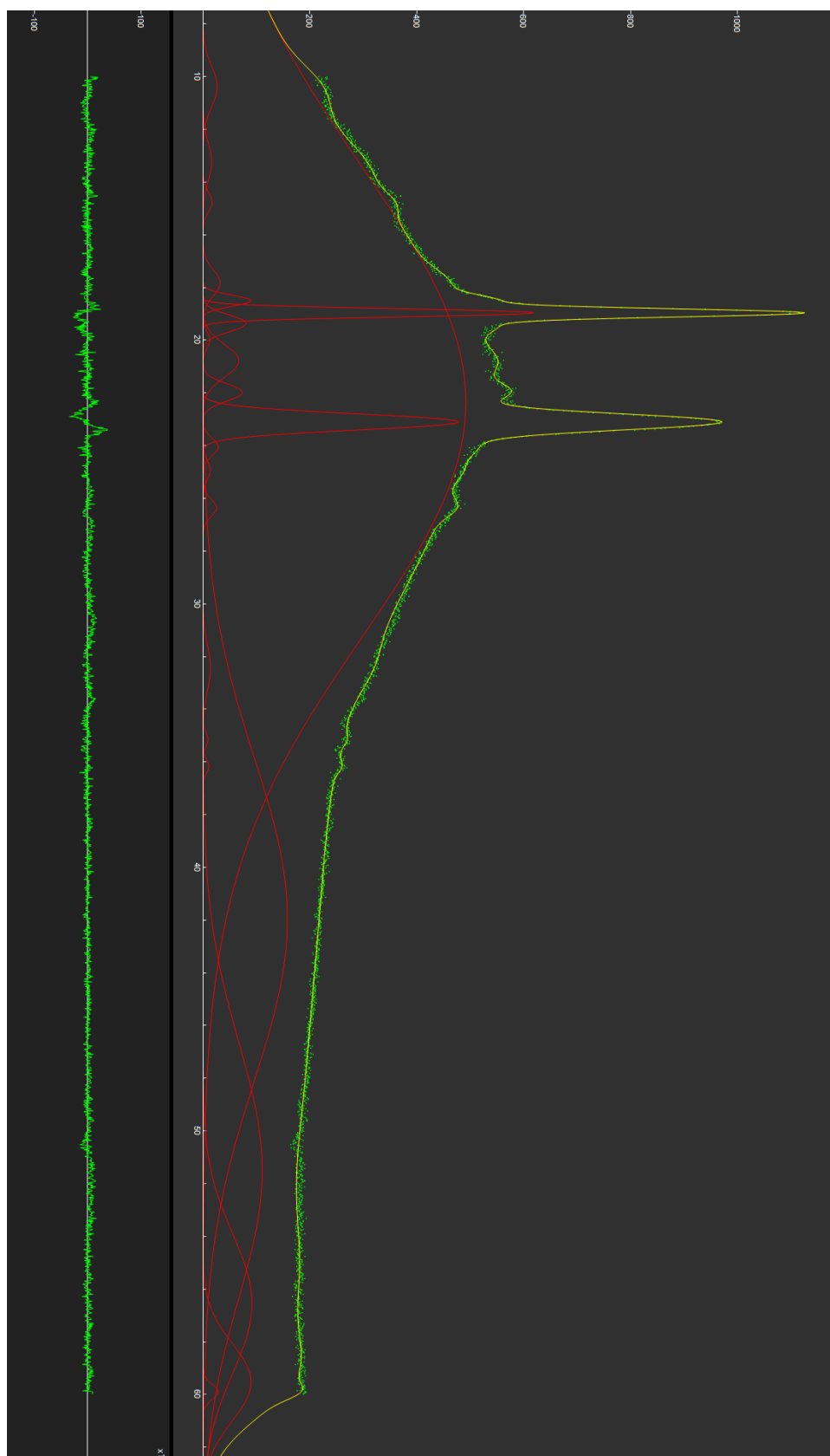
Figure 64. XRD deconvolution of hot stage sample: sample processed at 55 C and 20k lb f , run at 75 C.
