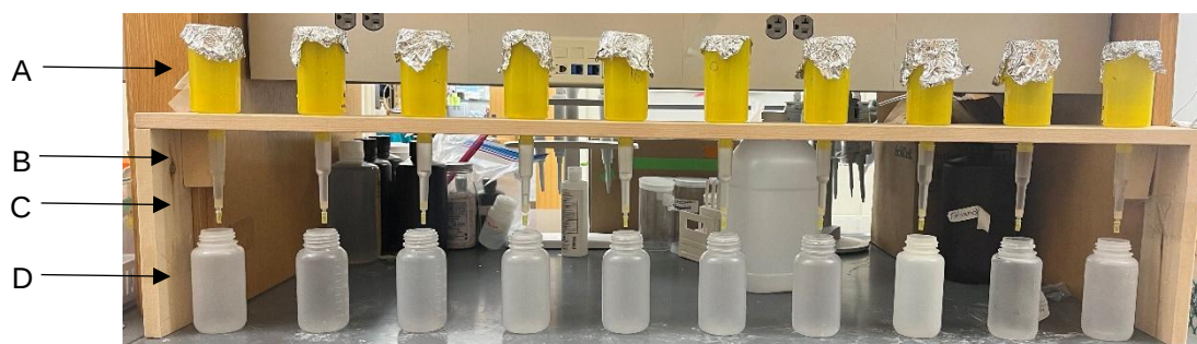
Figure 6: an image of the lab setup of the cation exchange resins. 10 separate resins were capable of being used at a time and could be flushed in between samples (e.g., they were reusable). A: funnel where eluent and filtered water was introduced, B: detachable column where sample was introduced, C: cation exchange resin that captured the \text{NH}_4^+ and removed anions and organics, D: waste containers that were switched out with vials when it was time to collect the purified \text{NH}_4^+ .
