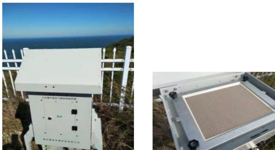
Figure 5: Left: An image of the high-volume aerosol sampler at Changdao Island, which operates at 1.0 \text{ m}^3/\text{min} (e.g., pumps the surrounding air onto the filter). Aerosol samples (bulk total suspended particles) were collected on pre-cleaned TE-G653 Glass Fiber Filters. Right: an example of a filter that has been collecting aerosols for 48 hours (filters started off white).
