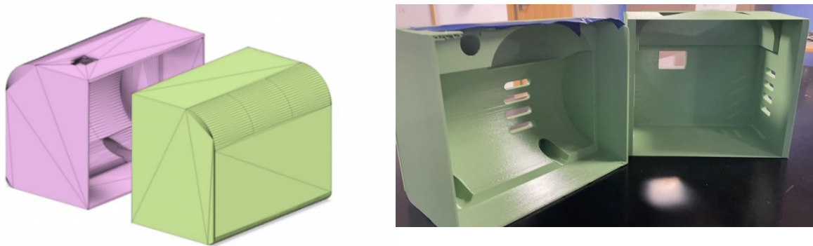
Figure 10 3D printed carrier (A) Design for fitting the carrier together (B) Printed carrier slots to allow the tubing, ventilation, and canister to sit within.
