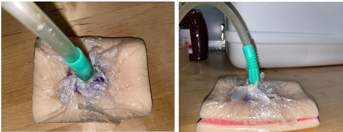
Figure 12 Silicone sponge model that was soaked in water. The tip was attached to the model using Seram to ensure a tight seal. This was further confirmed by the compression of the entire model due to the negative pressure environment.
