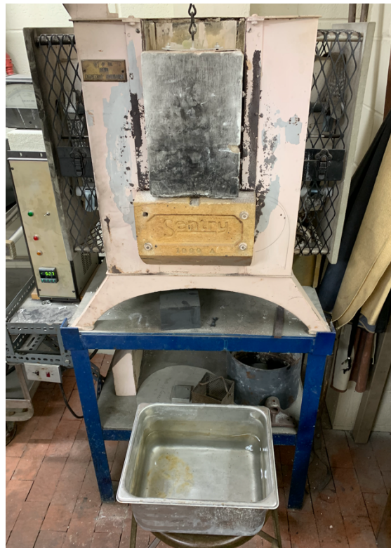
Figure 8. The furnace under the Prince Laboratory at Brown University. The molds displayed in figure 7 were heated in this furnace at 500°C for 60 minutes and quenched in water in the steel tub displayed.
