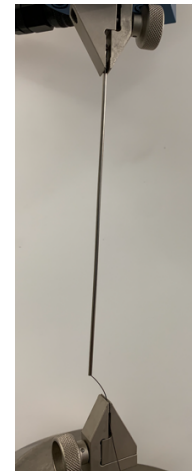
Figure 15. This figure displays the friction test that was conducted on the MTS machine for 0.4 mm nitinol austenite in a trained S-shaped zig zag geometry under 35 °C heat within a steel sheath. The maximum force recorded can be assumed to approximate how much force would be required to remove the sheath from the nitinol when in the body. This test was also conducted for a FEP and PTFE sheath.
