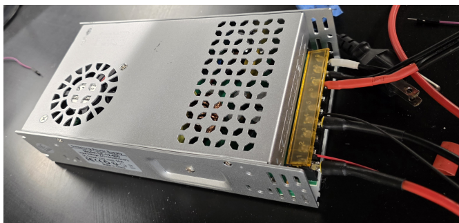
Figure 10: Switching DC power supply used to provide electrical power to the ESC array through the terminal-based distribution system.
