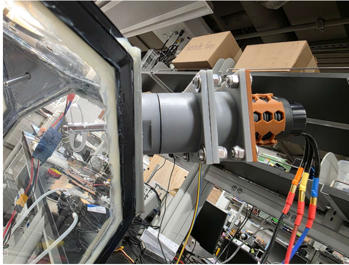
Figure 5: Representative installed corner-mounted drive unit after fastening to the chamber support structure.
