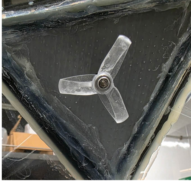
Figure 6: Three-blade impeller mounted on the exposed shaft inside the chamber.
