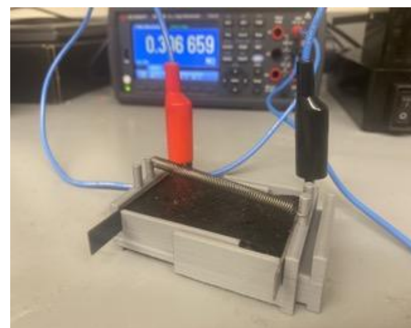
Figure 3. 3D printed static resistance testing apparatus in use while connected to multimeter.
