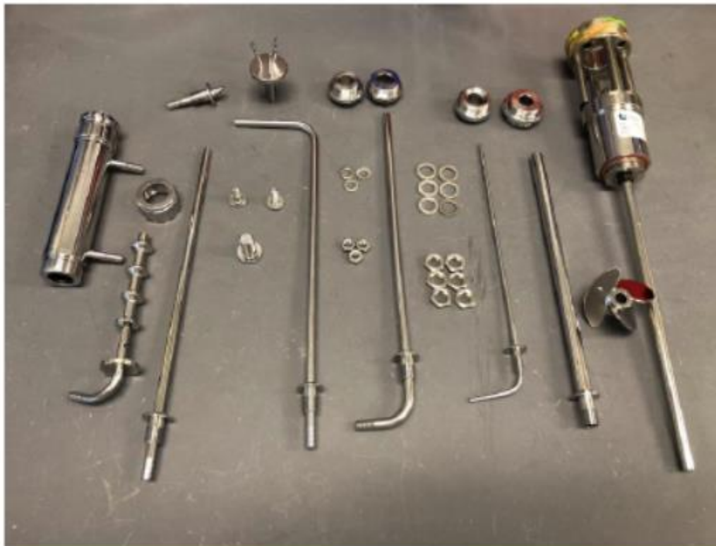
Figure 6; Bioreactor head plate parts
